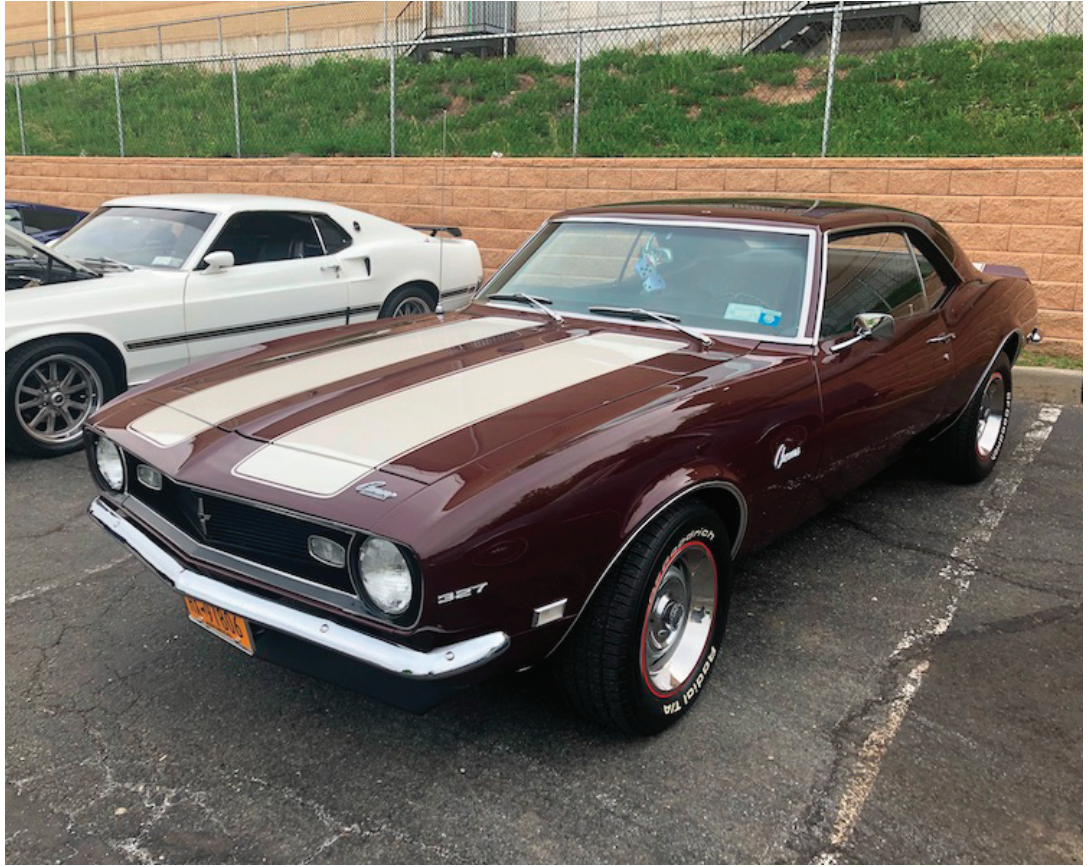
1968 Camaro also saw the switch from a circular to a rectangular side view mirror, and the placement of engine size emblems on the front of the fenders. Inside, much of the bright trimwork was changed to a brushed finish to reduce driver glare. (Photo by Paul Jr.)
