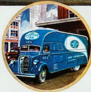
Studebaker Cab-Forward efficiency is most evident in cramped quarters, where the saving of upward of 40 inches in overall length saves hundreds of minutes and gallons of fuel in daily maneuvering.
