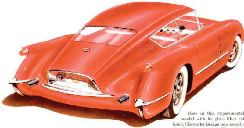
Here in this experimental two-passenger model with its glass fiber reinforced plastic body, Chevrolet brings new aerodynamic design to the closed sports car. The ultra-streamlined top sweeps back to a jet exhaust-type rear opening.
