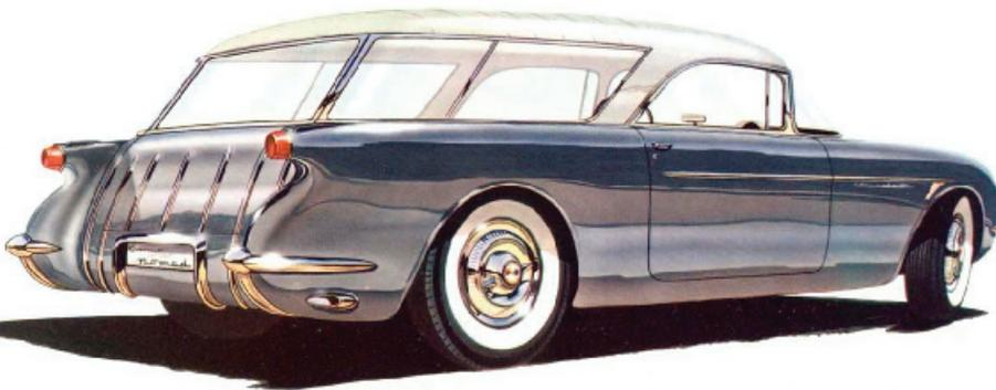
Here for the first time is an experimental model combining the sleek styling of a sports car with the versatility and utility of a Station Wagon. The glass fiber reinforced plastic body affords unusual visibility with seating
