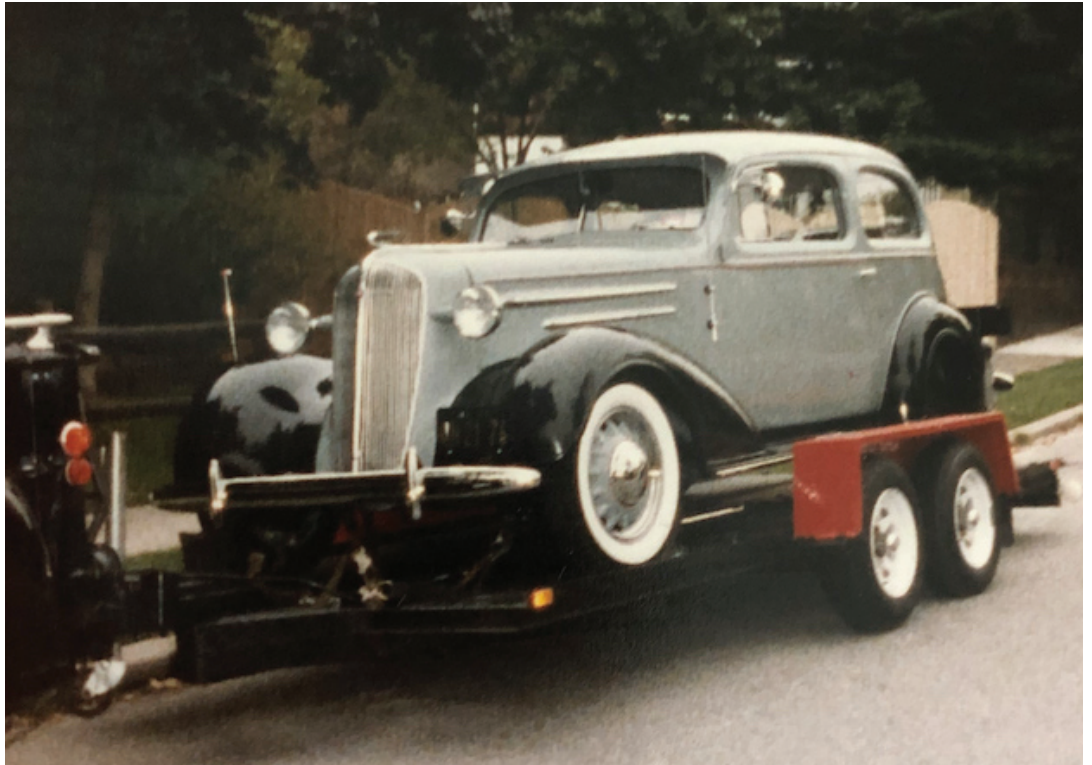
All 1936 Chevrolets were powered by an OHV inline six good for 79 horsepower. The 1970 Power Wagon most likely put out three times as many horses, giving Phil's Chevy one helluva ride (photos by Paul Jr.)
