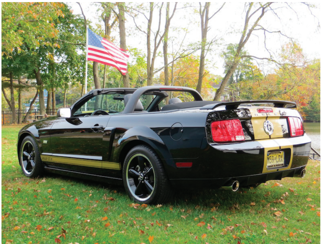
Shelby's GT-H features a new lowered suspension, free flow exhaust with X-pipe, cold air intake and a special computer chip, boosting the stock GT engine output to 325 HP. They also added a roll bar, front tower braces, a fiberglass hood, unique 18" wheels and gold stripes. (photos by Kevin Keenan)
