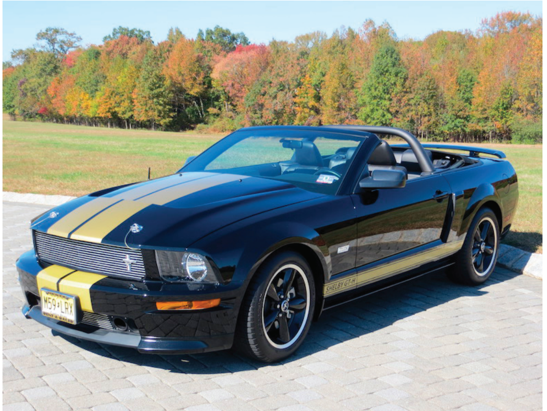
Shelby's GT-H features a new lowered suspension, free flow exhaust with X-pipe, cold air intake and a special computer chip, boosting the stock GT engine output to 325 HP. They also added a roll bar, front tower braces, a fiberglass hood, unique 18" wheels and gold stripes. (photos by Kevin Keenan)
