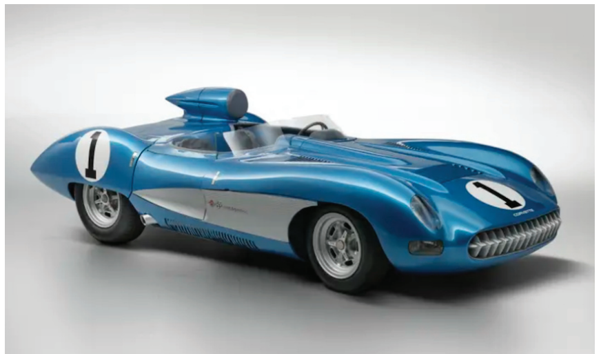
This was the first purpose-built GM factory racecar. It is powered by a Chevrolet 283 with Ramjet fuel injection, and features lightweight magnesium bodywork. Unfortunately, the body conducted heat directly into the cockpit, and the drivers could not bear the high temperatures. (photo by shooterz.biz courtesy of RM Sotheby's)
