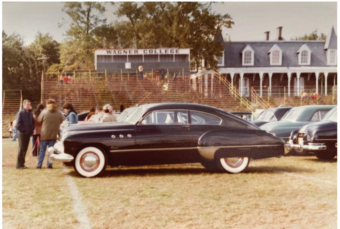
1949 marked the debut of Buick's VentiPorts. Those on early '49's are actually vents, but they soon became closed off ornaments. The Super featured three per side, while the Roadmaster had four.
