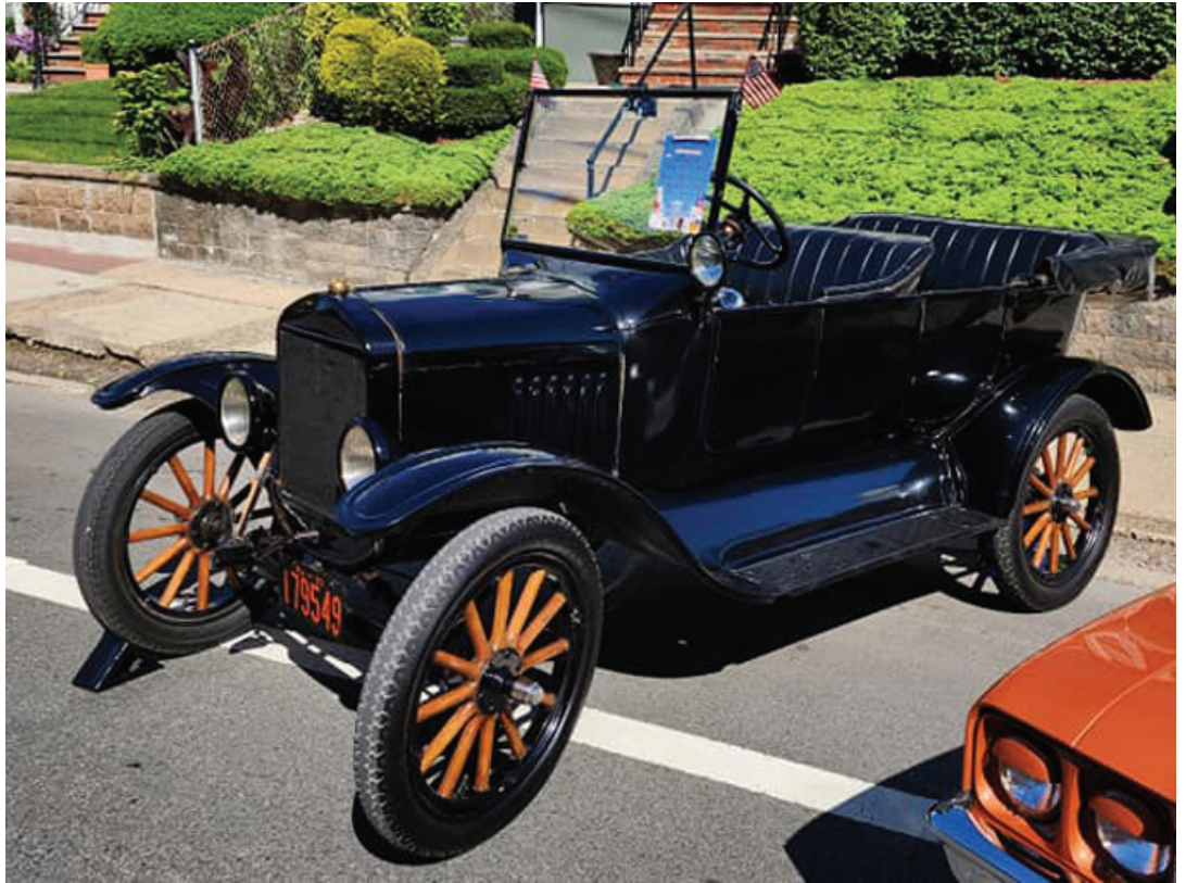
All Model T's were offered only in black from 1914 through 1925. In late 1926, open cars were offered in Phoenix Brown or Gunmetal Blue. Driving one is unlike driving other cars, as the throttle is controlled by hand, and reverse is controlled by foot. (photo by Enrico Ferrara)
