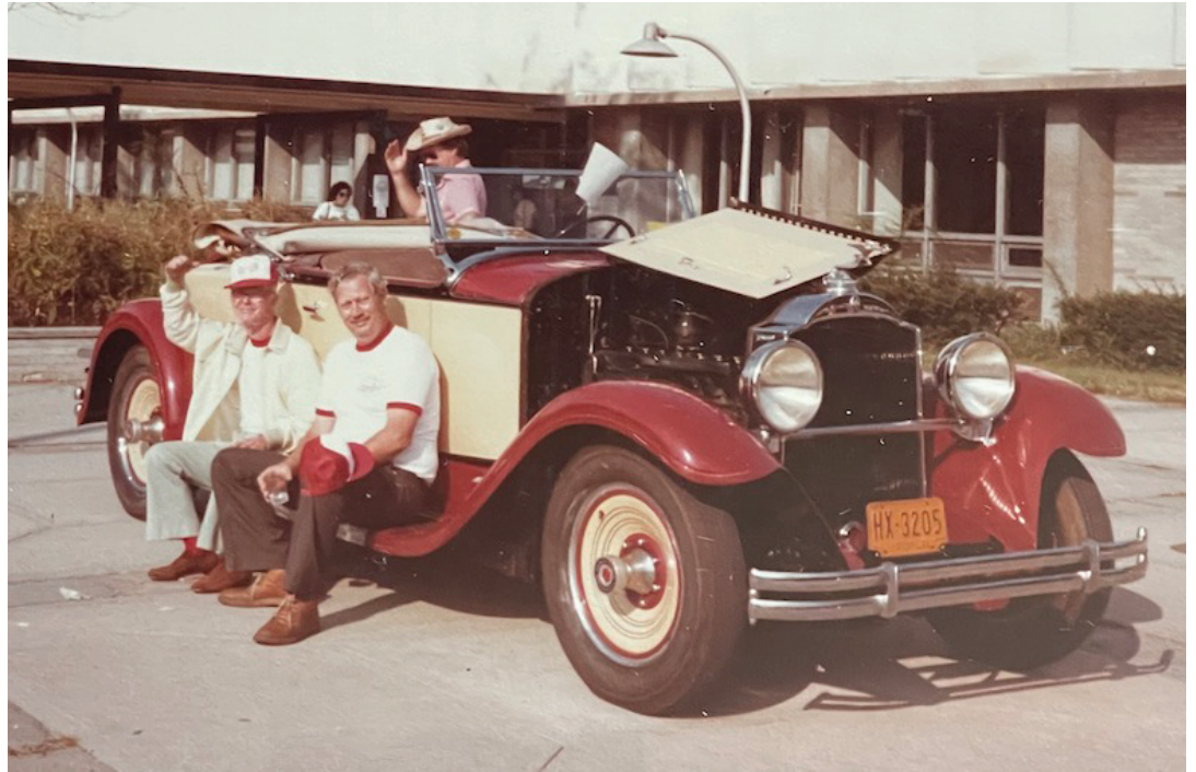
Former members Birger Nilsen (no hat) and John Fleming (wearing hat). Disc wheels were standard,, wire wheels were optional. 1931 steering wheels dropped one of the four spokes. (Photo by Sal DeFrancesco)
